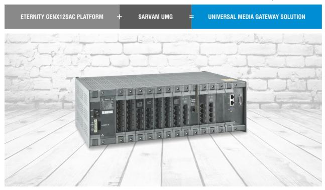
**ETERNTIY GENX12SAC**: It is a next-generation platform with CPU Card, 12 Universal Slots, and AC power supply in 19inch 4U enclosure. SARAVAM UMG with ETERNITY GENX12SAC encompasses functionality of IP at core, offering high-density VOCODER (VOIP) channels through DAUGHTER-BOARD MODULE (NX DBM VOCODER64) which can be availed in steps of 4/16 VOCODER channels licenses as per simultaneous VOIP calls requirement.
