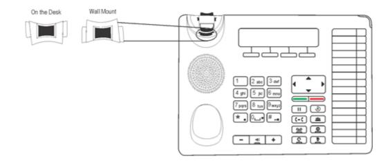
If you are unable to remove the wall mount tab, you may use a tool like a minus screw-driver to remove it.
