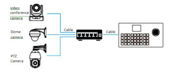
(2) Analog mode RS 485 control camera connection diagram.
