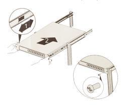
• You can use Round Hole pins or Square hole pins. Align the holes of the system with those of the rack and insert the screws. Tighten them to fix the system in place.
